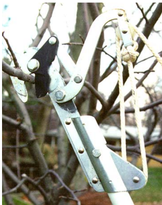
Tree trimmer. The four bar linkage is a double lever mechanism used to increase the mechanical advantage
